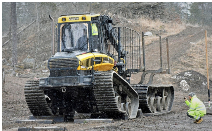
Figure 2. The constructed machine traversing Skogforsk's vibration test track (photo: Rolf Björheden).
