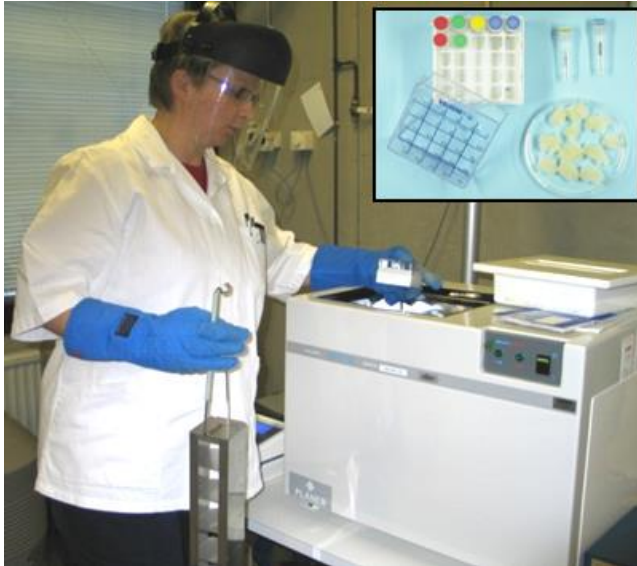
Slow-cooling of SE samples in programmable Planer device and in Mr. Frosty was compared
